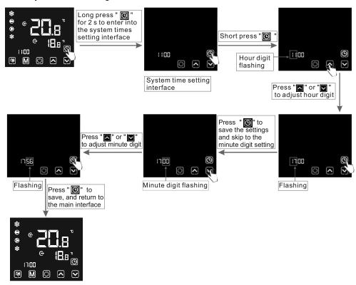
Notes: Under the clock setting interface, if there is no operation for 20 s, the system will automatically memorize use's settings, and return to the main interface; if short press "U runing any operating steps, the changes will not be saved and return to the main interface.
