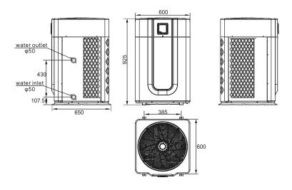
Model:PV 21/PV 24 unit mm
